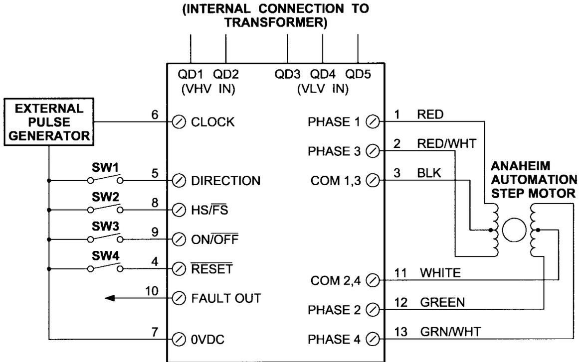
Figure 5: Typical Hook-Up for Clockwise and Direction Option and Motor Wiring.
