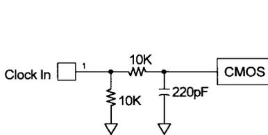
Figure 2: Positive Going Clock Input
