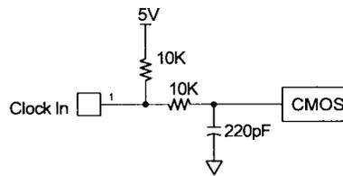
Figure 3: Negative Going Clock Input
