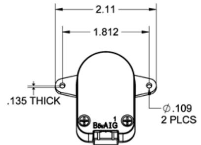
G-Option: Includes molded ears which enables it to be mounted to a 1.812" diameter bolt circle. Mounting holes are designed to fit 4-40 screws. Will work with shaft lengths of .445" to .570" and does not add to the required shaft length.
