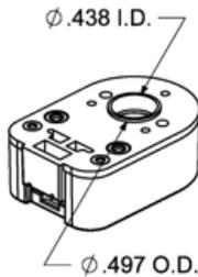
A-Option: Adds a .497" diameter alignment shoulder designed to slip into a .500" diameter recess in the mounting surface centered around the shaft.
