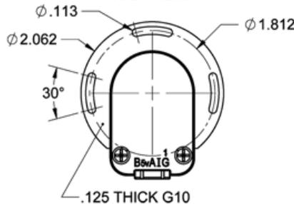
R-Option: Adapter is an 1/8" thick fiberglass adapter which is pre-mounted to the base of the encoder. It allows the encoder to rotate +/- 15 degrees.
